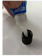
6. Press the knob onto the insert with the pointer located well above the fully counterclockwise pointer position. Skirted knobs do not have pointers.
