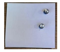
8. Rotate the knob counterclockwise until the pointer aligns with the position indicated by the template. This step is not required for skirted knobs.
