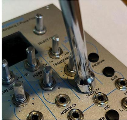
4. Remove the nuts beneath all 7 knobs with a 10mm nut driver. Be very careful not to scratch the panel during this operation. Covering the nut driver with heat-shrink tubing can be helpful. The skirted knob will not have a washer under the nut, the non-skirted knobs may or may not have one. The washers under the non-skirted knob are not necessary.
