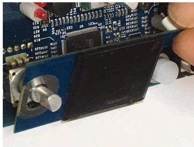
9. Pull on the sides of the flat cable connector lock to unlock the connector, and pull out the flat cable and remove the failed OLED Display PCBA. (The locking piece may be either white or black in color; black is shown here.)
