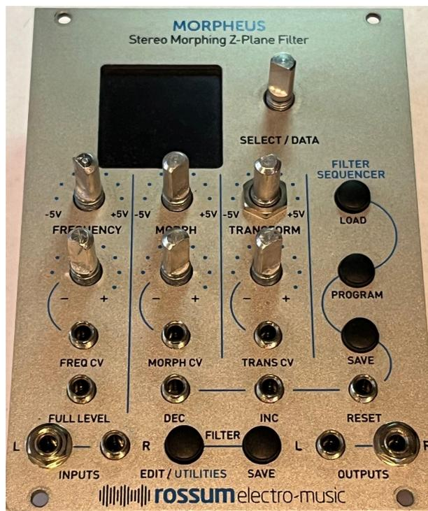
19. Now power up the Morpheus and check the module to make sure there are no issues and that the new OLED Display works and is visually level.
