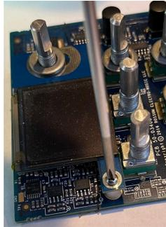
8. Fold OLED Display PCBA up from the encoder.
