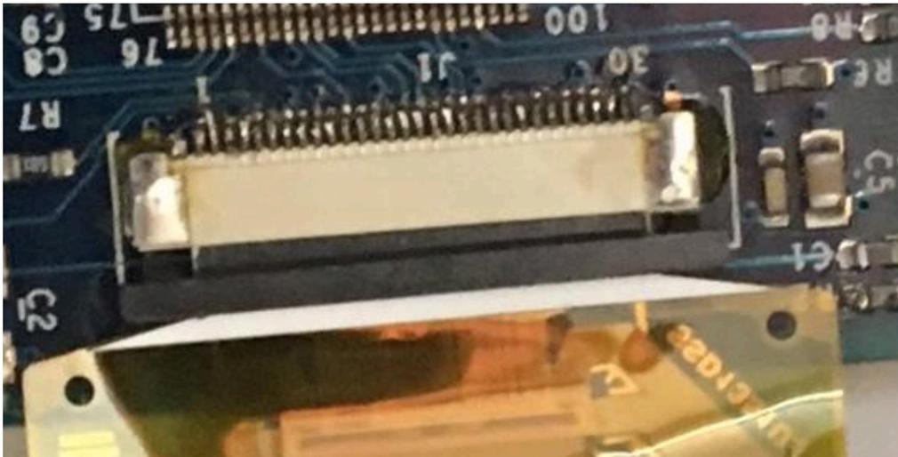
12. Carefully push the connector lock into the locked position, leaving the flat cable completely seated and the white cable area parallel to the connector.
